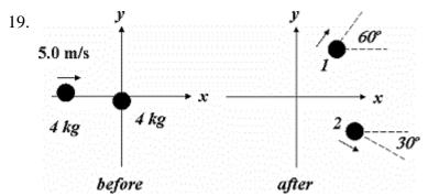
An inelastic two-dimensional collision between two objects of equal mass occurs as shown in the figure. What is the speed (in m/s) of the object moving into the first quadrant, the one labeled "1"?
