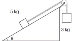
The coefficient of static friction between the block and the inclined plane in the figure is 0.20. What is the least angle  $\theta$  at which the blocks will remain stationary?
